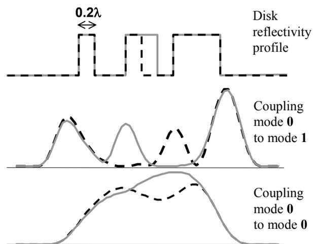
**Figure 2a: Two bit pattern with bit length  $0.2 \lambda$**
