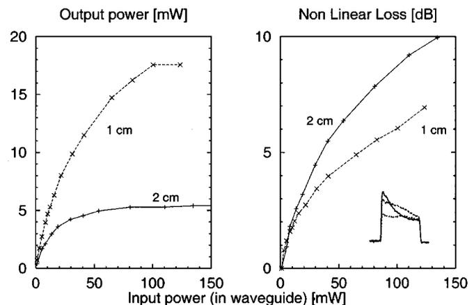
Fig. 1. Measured output power (left) and nonlinear loss (right) versus input power for a rib-loaded InP–InGaAsP passive waveguide ( $W = 2.5 \mu\text{m}$ ). The inset shows the transmission of a 4-ns square pulse for increasing input power ( $P_{\text{in}} = 10, 35, 70 \text{ mW}$ ).
