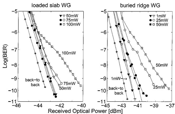
Fig. 4. BER measurements for a rib-loaded (left) and a buried ridge waveguide (right). Closed (open) symbols are for single- (two-) channel operation. The denoted powers are the total power coupled into the waveguide (sum of both channels).
