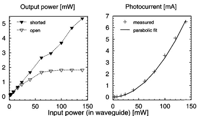
Fig. 5. Transmission results (left) and generated photocurrent (right) for a buried ridge waveguide with a p-n junction ( $\lambda_g = 1.3 \mu\text{m}$ ).
