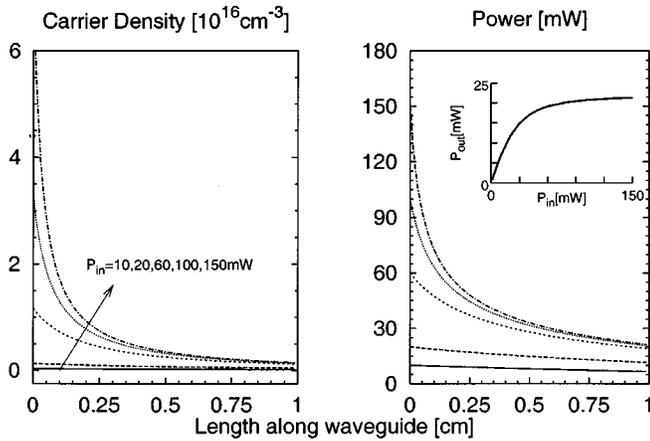
Fig. 2. Simulated carrier generation (left) and power evolution (right) along the waveguide ( $\beta = 60$  GW/cm,  $\tau_e = 4$  ns,  $A_{\text{eff}} = 1.7 \mu\text{m}^2$ ,  $L = 1$  cm,  $\alpha = 1.5$  dB/cm). Inset of right picture shows the output power as function of the input power.
