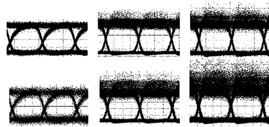
Fig. 3. Eye diagrams (2.5 Gb/s) measured from the output of a  $1.2\text{-}\mu\text{m}$ -wide buried ridge waveguide. Upper row: single channel in waveguide. Lower row: two channels present in waveguide. The second channel is filtered out using a bandpass filter before measuring the eye diagram. Left to right:  $P_{\text{in,total}} = 1$  mW, 75 mW, 150 mW.
