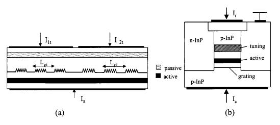
Fig. 1. Schematic structure of a  $\lambda/4$ -shifted (S)SG TTG laser. (a) Longitudinal/transverse cross section. (b) Lateral/transverse cross section.
