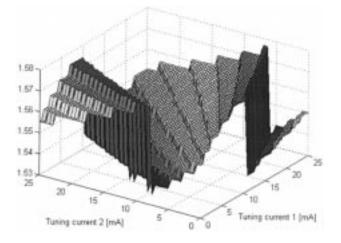
Fig. 2. Three-dimensional view of the wavelength (in  $\mu$ m) as a function of the two tuning currents.
