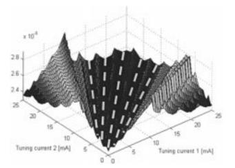
Fig. 4. Threshold gain  $(in \mu m^{-1})$  as a function of the two tuning currents. The dashed lines indicate lines along which a minimum gradient in threshold gain is obtained.
