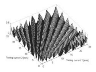
Fig. 3. Normalized threshold gain difference  $(\Delta(\Gamma g_{tln}L))$  between main and sidemode as a function of the two tuning currents.
