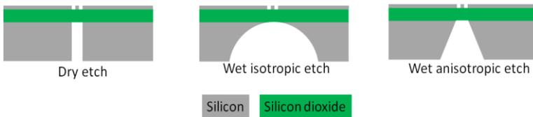
**Figure 3.5:** Schematic of dry etching (left), isotropic wet etching (middle), and anisotropic etching (right) of Silicon.
