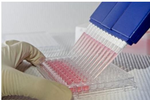
**Figure 1.2:** A microtiter plate is a standard tool in biomolecular research, and consists of small wells in which assays such as ELISA can be performed.
