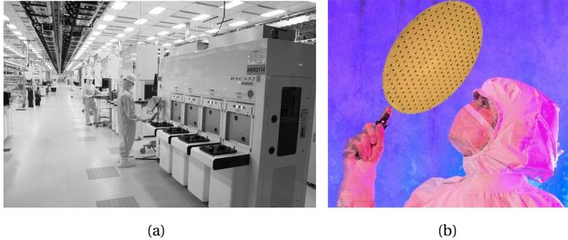
**Figure 1.5:** High-quality silicon photonic chips can be manufactured using the facilities already invested in by the electronics industry (a), providing the means to fabricate them at wafer-scale (b) in high volume at a low cost per chip. Images adopted from the IBM-website [31]
